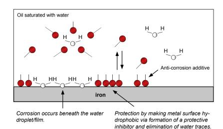
Alkali, Metal or Alkanolamine salts of ADDAPT PEX™ are suggested as corrosion inhibitors for (multi) metal protection. ADDAPT Chemicals offers a comprehensive range of formulated corrosion inhibitors for this purpose.
