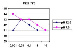
**Note:** x-axis = concentration / y-axis = Static Surface tension-Dynes.cm-2
