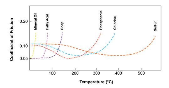
The proper choice of PEX™ phosphate ester offers an environmentally safe alternative to Cl-paraffins. They can be used in all Metal Working Fluids:
